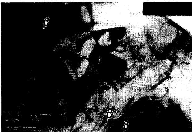
Fig. 3. TEM image of elongated \beta -sialon grains without cores.
